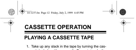
Take up any slack in the tape by turning the cassette's hub with a pencil. Do not touch the exposed tape.
